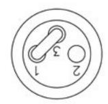
The amplifier can be driven single-end or balanced, if driving the amplifier single-ended, leave the supplied jumper in place (between pins 1 & 3 on the XLR). Your amplifier will operate without the jumper in place, but performance will be significantly diminished.
